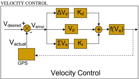
Velocity PID Control Loop. PID is a standard error driven control method.
