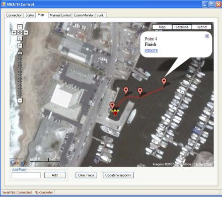
**Google Maps Interface.** Using C# hooks into javascript, Google Maps was able to be utilized for real time monitoring and waypoint routing for the autonomous SWATH boat.
