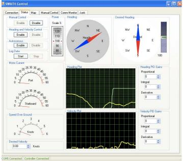
**Monitoring Graphical User Interface.** The graphical interface designed in Microsoft Visual C# allows monitoring and adjusting the boats performance, including tuning PID gains in real time.
