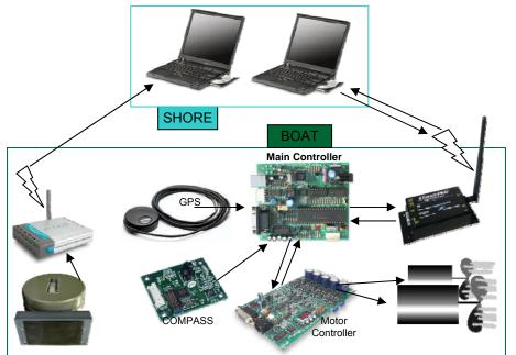
**System Diagram.** Arrows display serial communication directions among the various components of the system. Scientific instruments can be plugged in to a wireless Ethernet link and act as an independent system.
