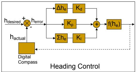
Heading PID Control Loop. PID is a standard error driven control method.
