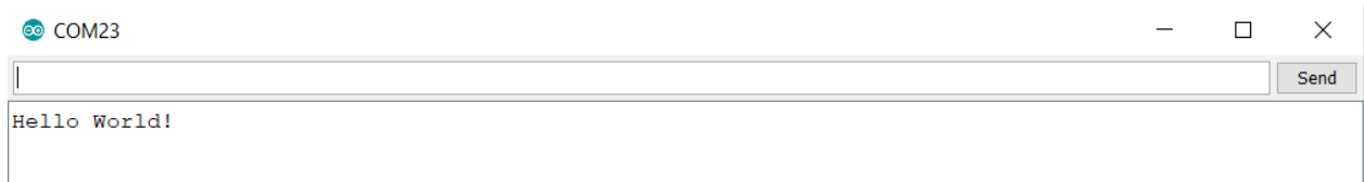
Figure 3: ‘Hello World’ text printed on the Arduino serial monitor. The text confirms successful communication between the board and your computer.
