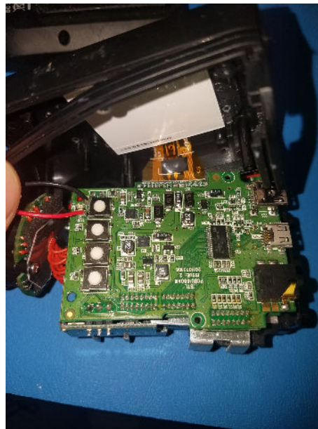
Figure 11: A Sony Drift HD camera with the main housing removed with wires soldered onto the sides of the 'play' button.
