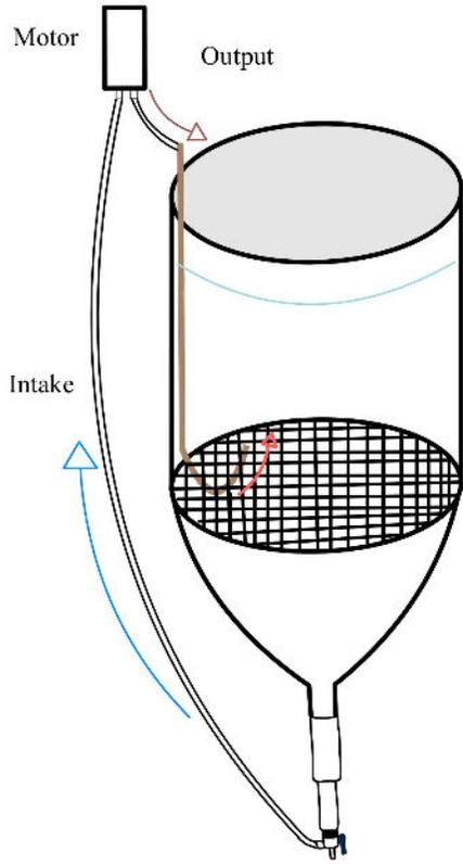
Figure 1: A simple schematic showing the general design of the tanks constructed for the trials
