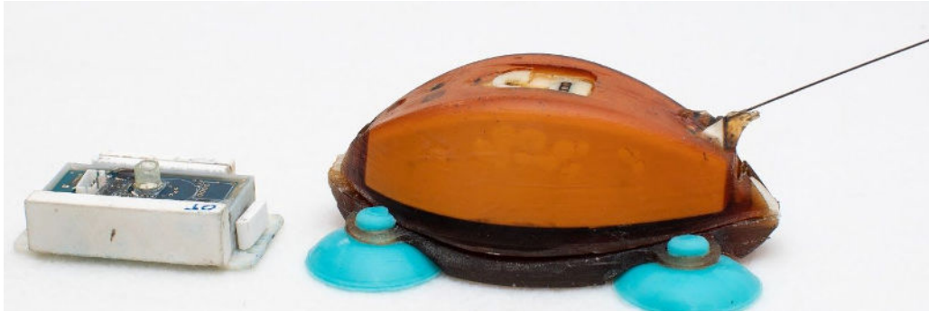
Fig. A: Shows the size comparison between the potted iTAG v0.4(left) & the iTAG v0.1(right). Although both versions are intended to be placed on the bell of a jellyfish, The v0.4 uses glue to remain affixed whereas the v0.1 uses suction cups.
