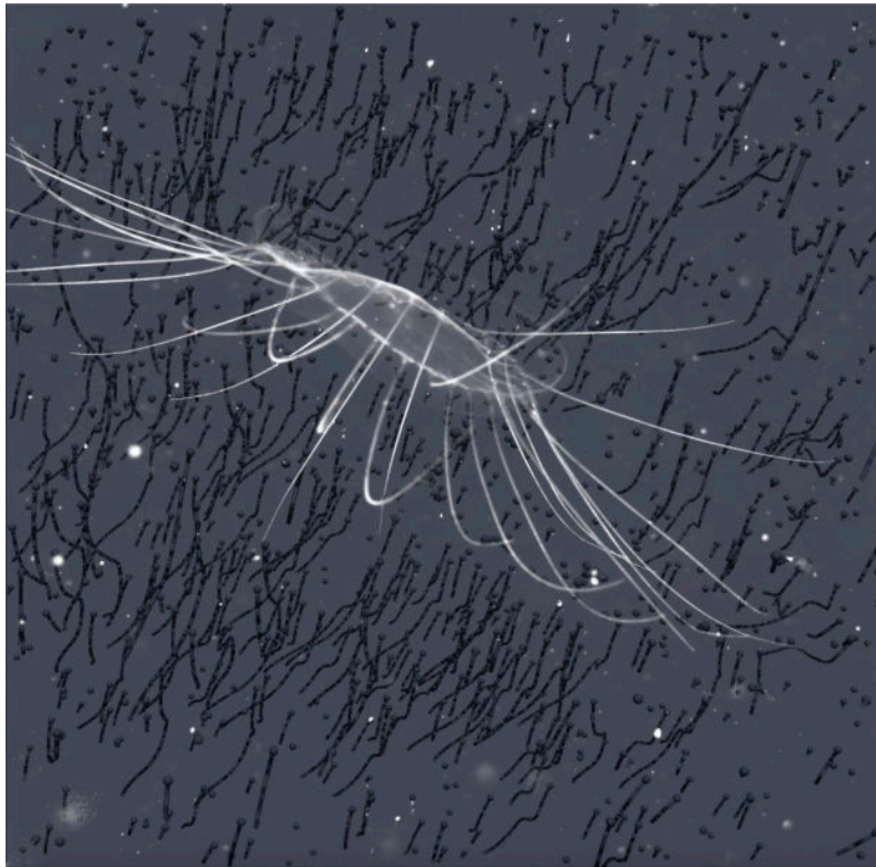
Figure 2: The final frame of the particle positions and trajectories overlaid onto the total focus video of the Solmissus clip of interest is shown. Note the grouping of particles within the top edge of the bell which were used to approximate the outer edge of the bell in creating the final streamline animation.
