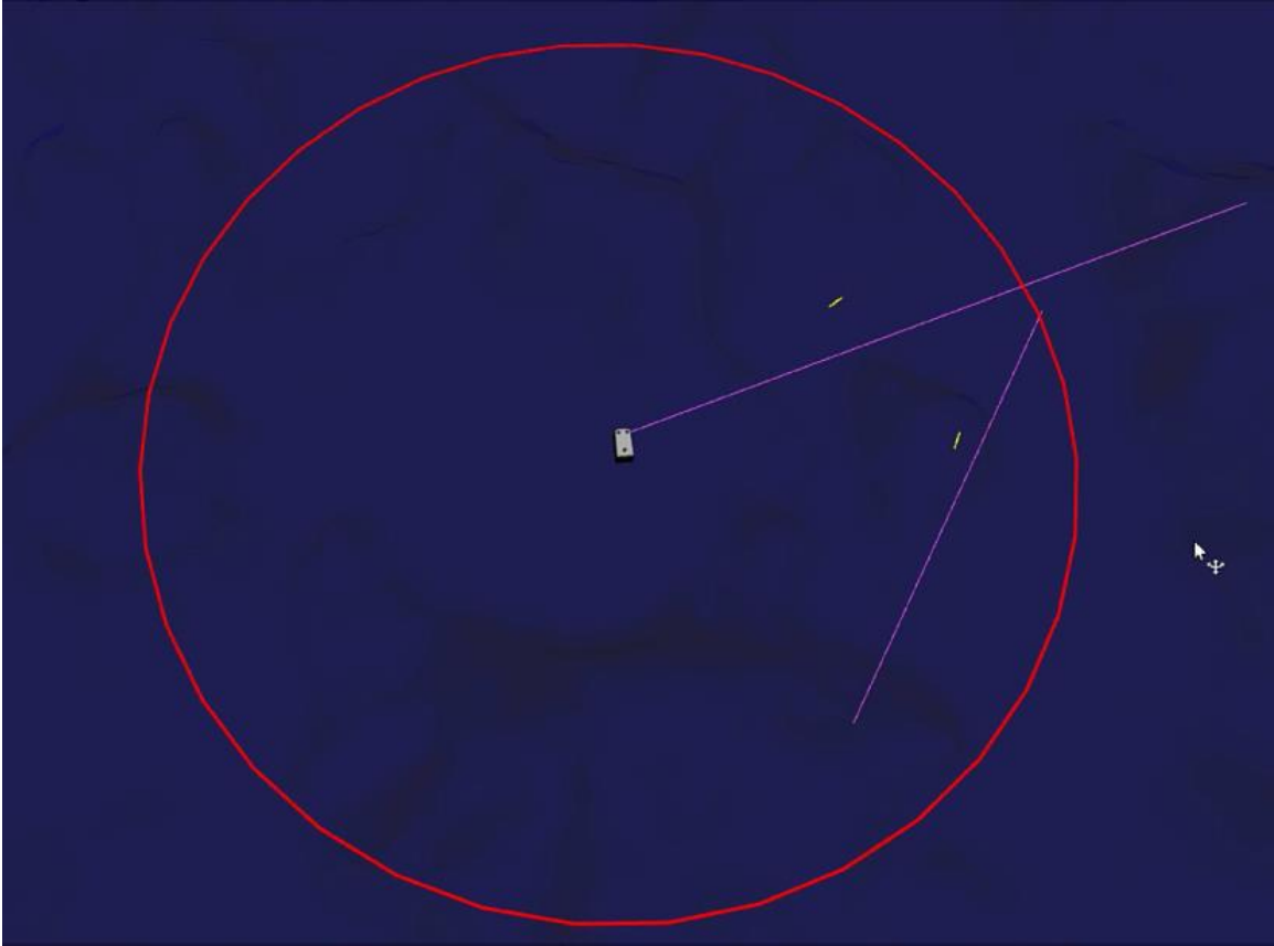
Figure 15: LRAUVs have gotten close enough to the Surface Station to split off into their individual behaviors. Circular yo-yo movement LRAUV is splitting off while the other LRAUV continues to the Surface Station.
