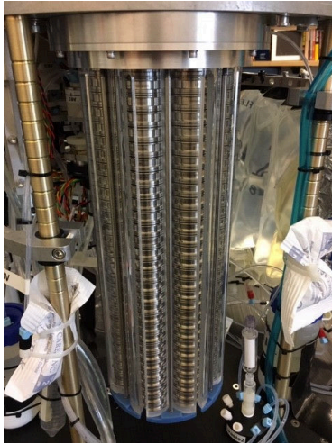
Figure 1. A syringe mechanism (top) in a 2G-ESP is used to draw water through the filters enclosed in metal chambers called pucks (middle). Once the lysate and preservative are added to the pucks, they are placed inside the tube (bottom).
