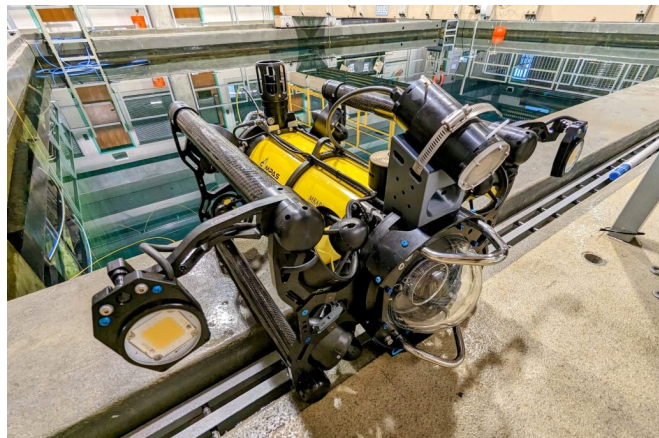
Fig. 1: This figure shows the MOLA AUV (the vehicle used for testing) sitting next to the test tank.
