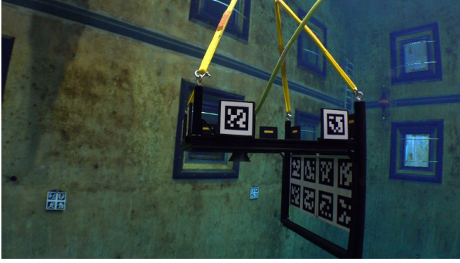
Fig. 3: This figure shows the prototype dock hanging in the test tank. Note the Apriltags on the dock and the test tank wall behind.
