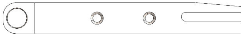
Figure 4: Top view of weight rod end showing release pin hole and half-slot
