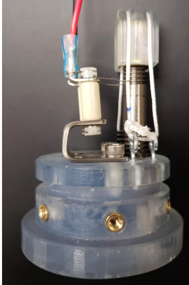
Figure 5: Assembled pin puller end cap
