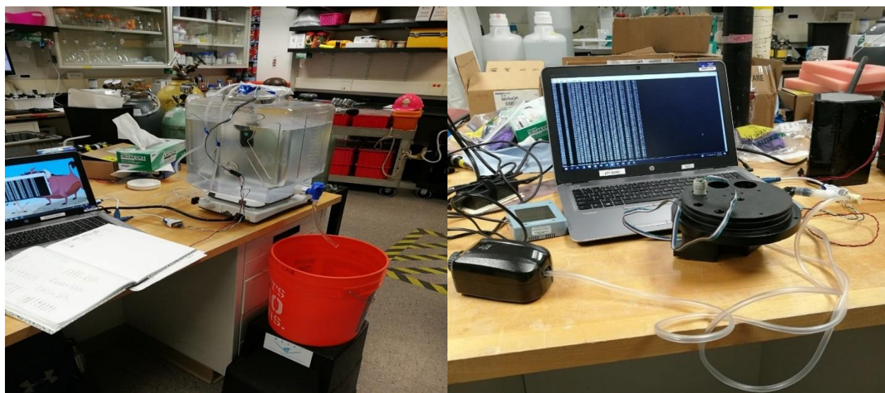
Figure 1: Depictions of lab-controlled calibration experiments consisting of Winkler-based calibration (left) and simplified air calibration (right).
