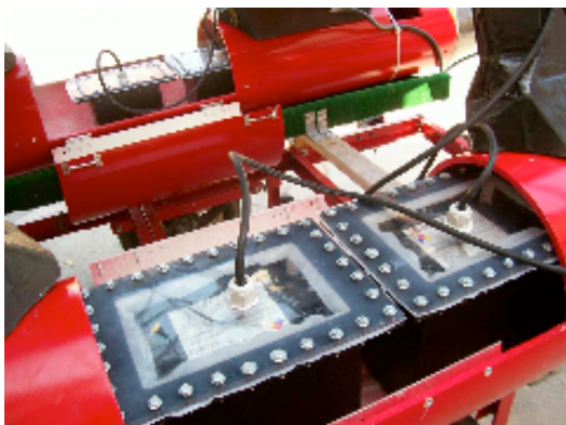
Fig. 3: Batteries installed in hulls watertight boxes
