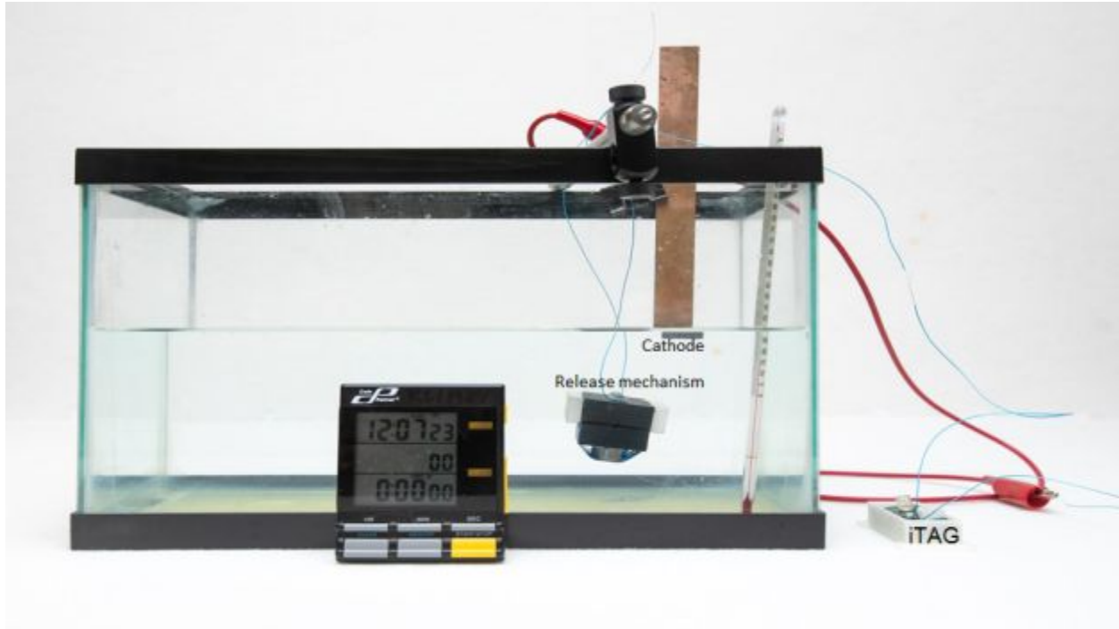
Fig 6: Shows the release mechanism setup. Connected directly to the iTAG, it can be pre programmed to a specific time for the release mechanism to activate. A multimeter(not pictured) shows the change in voltage once the switch is activated.
