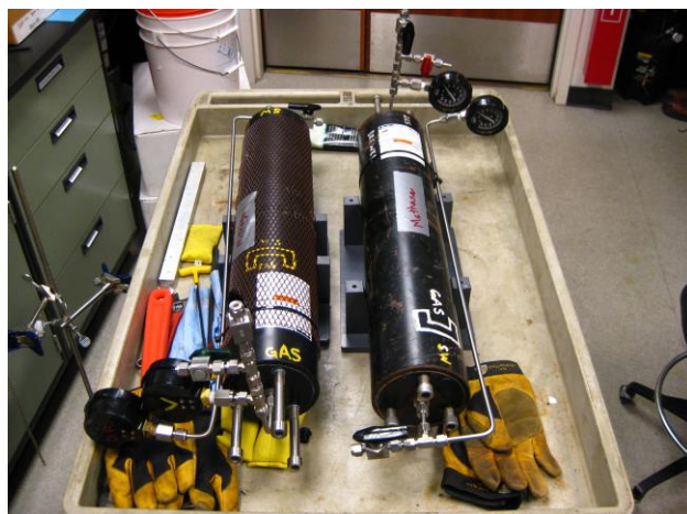
Figure 2: Piston accumulators like those used on the Doc Ricketts dive. One end is pressurized at the surface, then seawater is pumped in the other end at depth to create a pressure differential.
