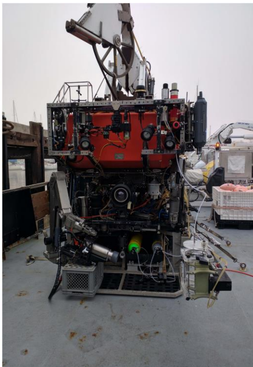
Figure 1: Various equipment used for spectra collection. a) The DORISS II system partially inserted into its pressure housing. b) The custom Adams & Chittenden glass D-sampler with perforated metal stage. c) The sampler and laser probehead mounted on the ROV Ventana . On the shelf are the two gas tanks used to bring Argon down to flood the sampler, and on the top right are the niskin bottles to collect the samples for lab use.
