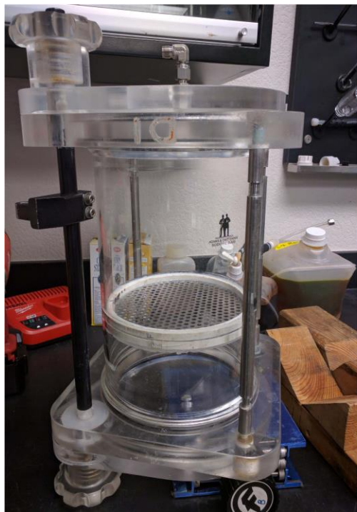
Figure 1: Various equipment used for spectra collection. a) The DORISS II system partially inserted into its pressure housing. b) The custom Adams & Chittenden glass D-sampler with perforated metal stage. c) The sampler and laser probehead mounted on the ROV Ventana . On the shelf are the two gas tanks used to bring Argon down to flood the sampler, and on the top right are the niskin bottles to collect the samples for lab use.
