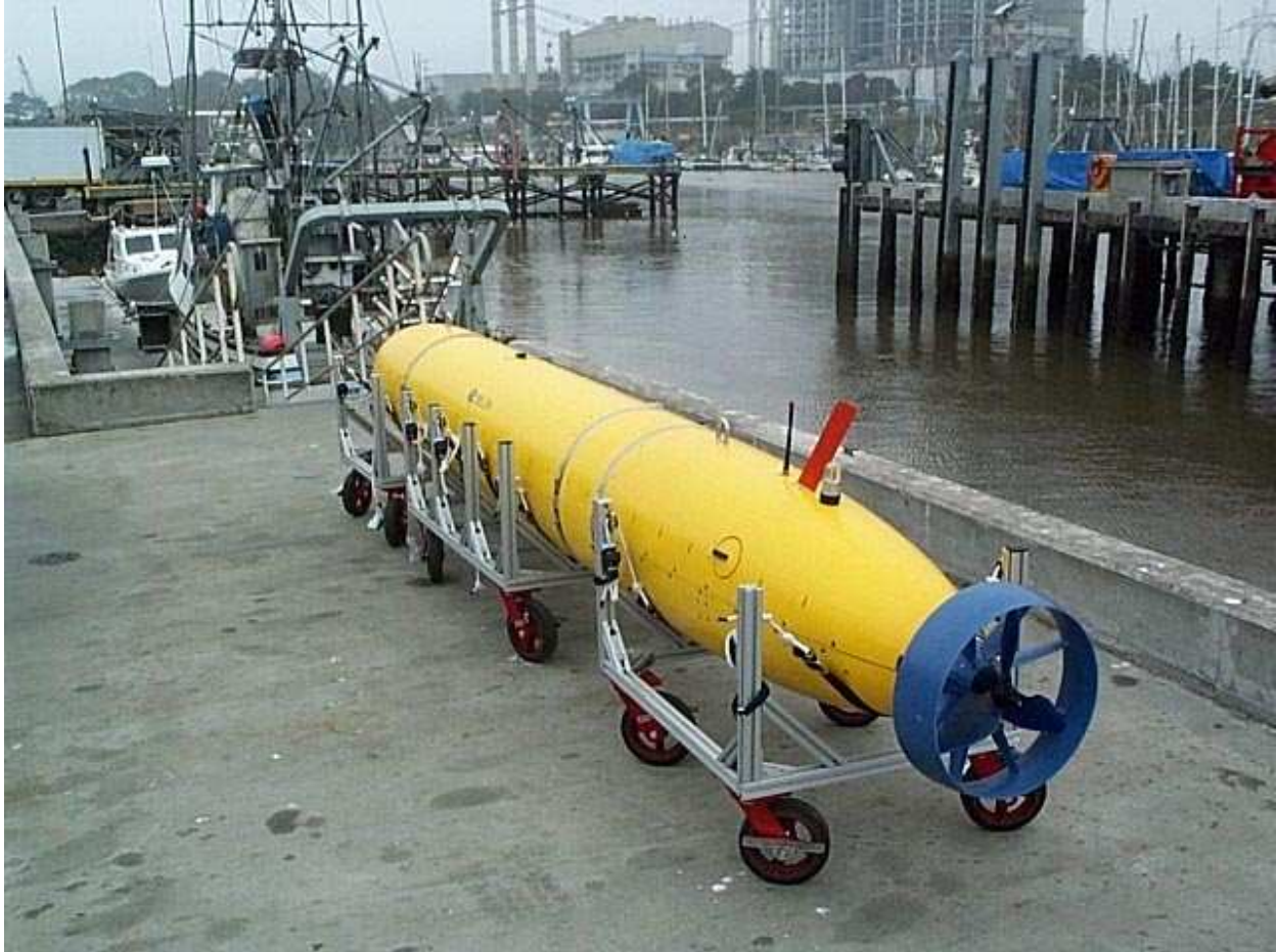
Figure 2: Ring-Wing and Propeller. Here there is only one 66 inch fuelcell midbody, and a 10 inch midbody for extra flotation, making the vehicle 419 cm in length. The vertical fin is the RF/GPS antenna.
