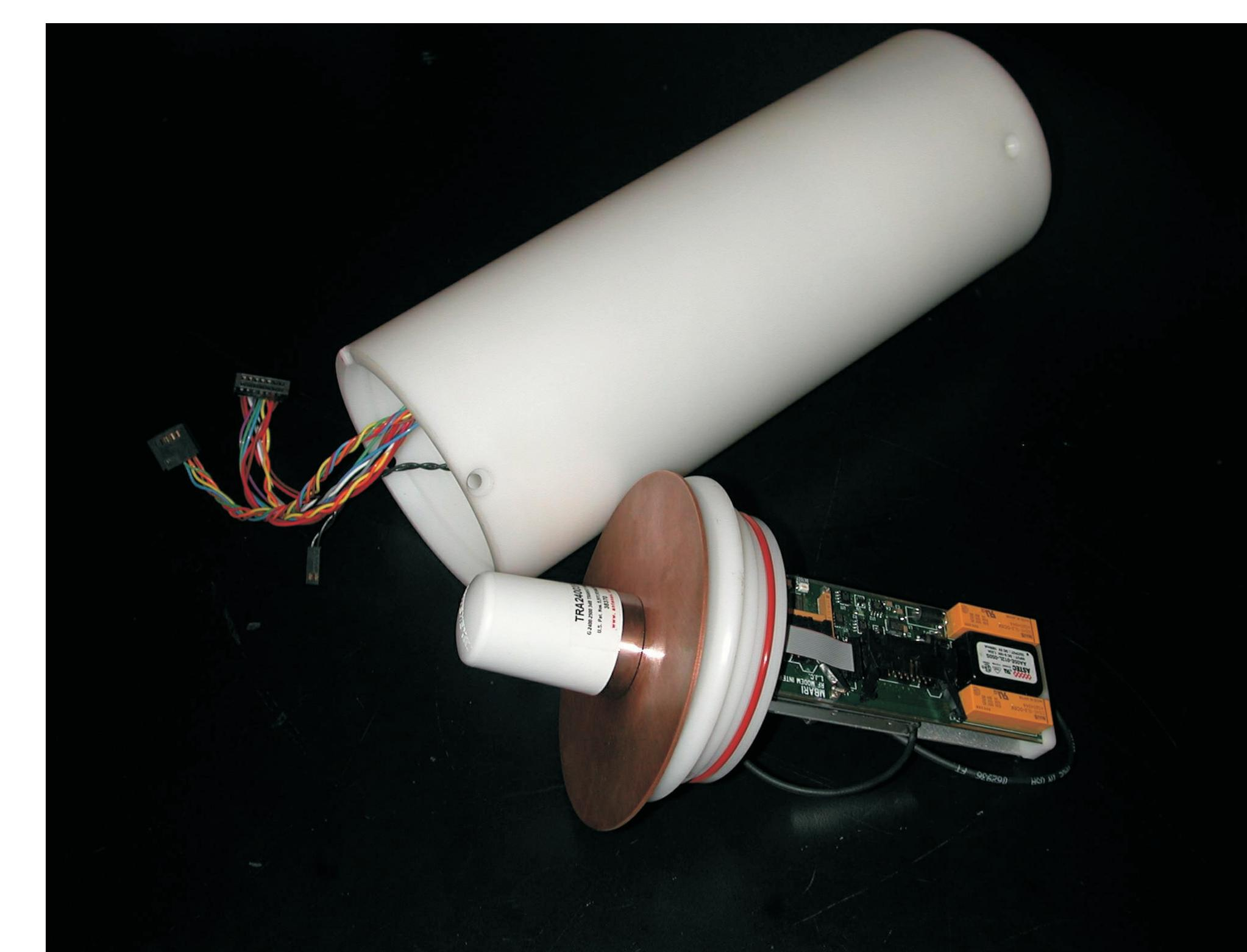
The LOBO radio assembly, shown above, incorporates a MBARI designed interface that provides electrical isolation between the LOBO datalogger and the Cirrionet WIT2410 Wireless LAN module. Electrical isolation of the data and control lines minimizes sensitivity loss in the radio due to conducted emissions.
