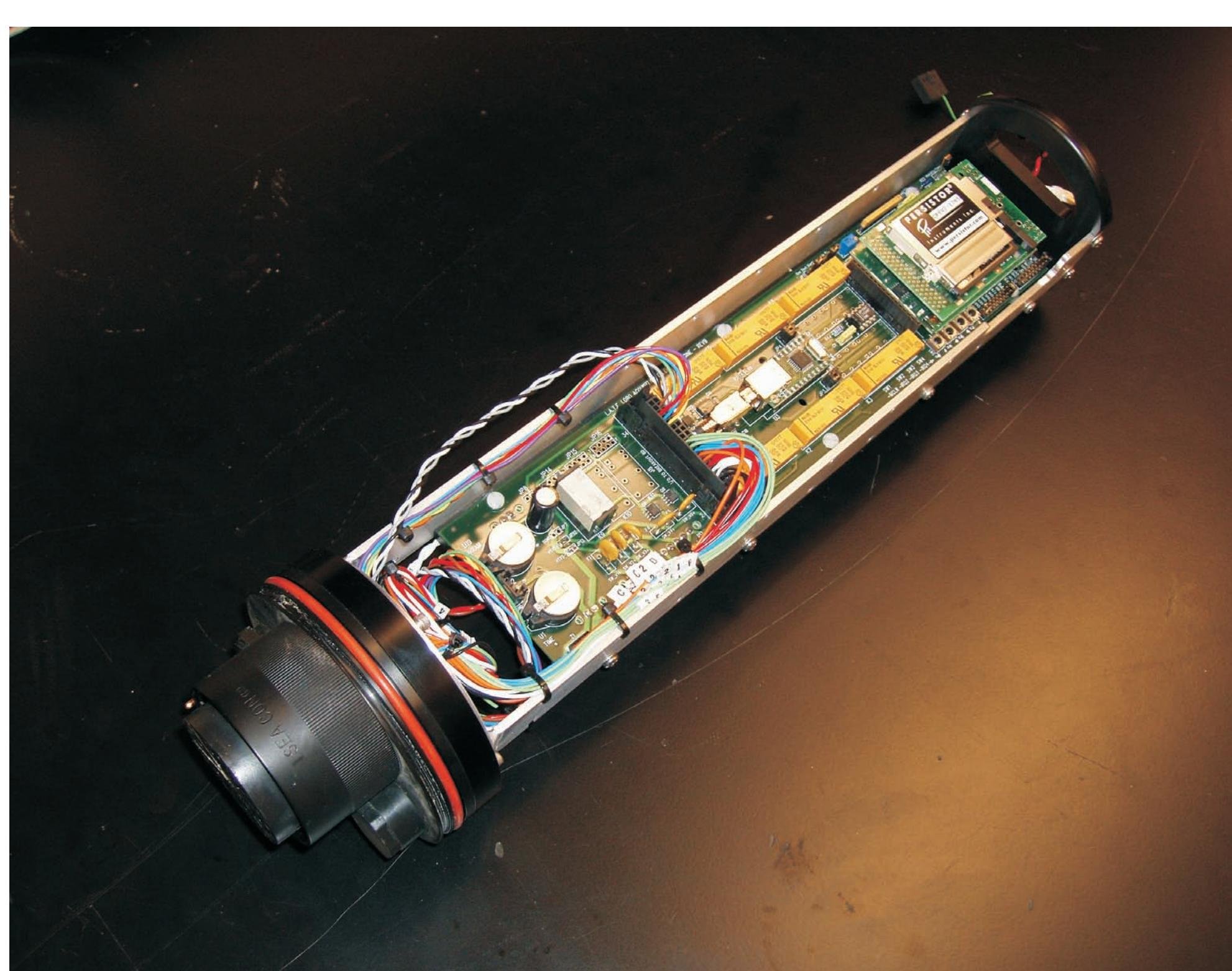
Instrument data is logged and telemetered by a MBARI designed datalogger, shown above. The datalogger can communicate with up to eight serial devices and transmit hourly for up to six months from a single battery pack.
