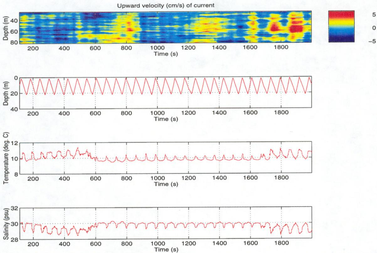
Figure 4. Earth-referenced vertical current velocity and CTD measurements.
