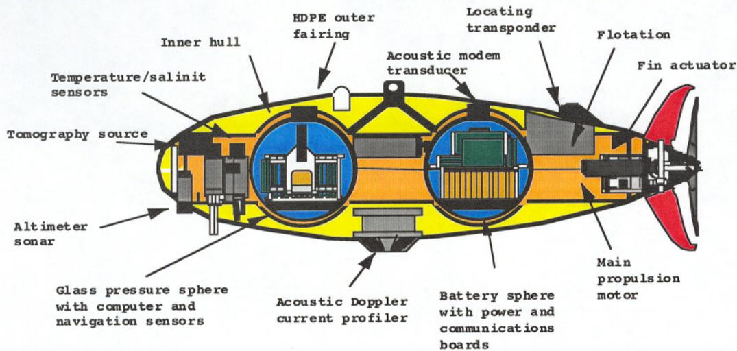
Figure 1. AUV Xanthos in its Haro Strait configuration with downward facing RDI ADCP in its midsection (courtesy of Dr. James Bellingham).
