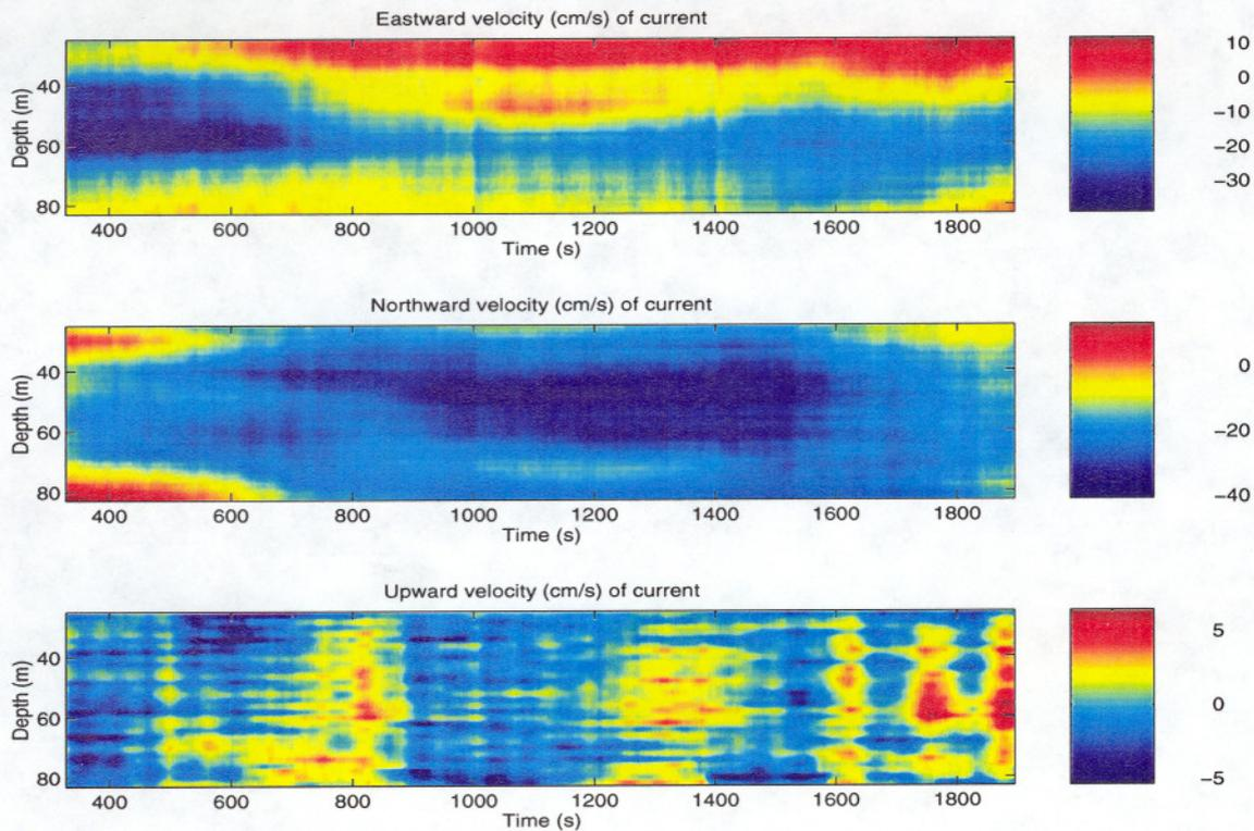
Figure 3. Earth-referenced current velocities.
