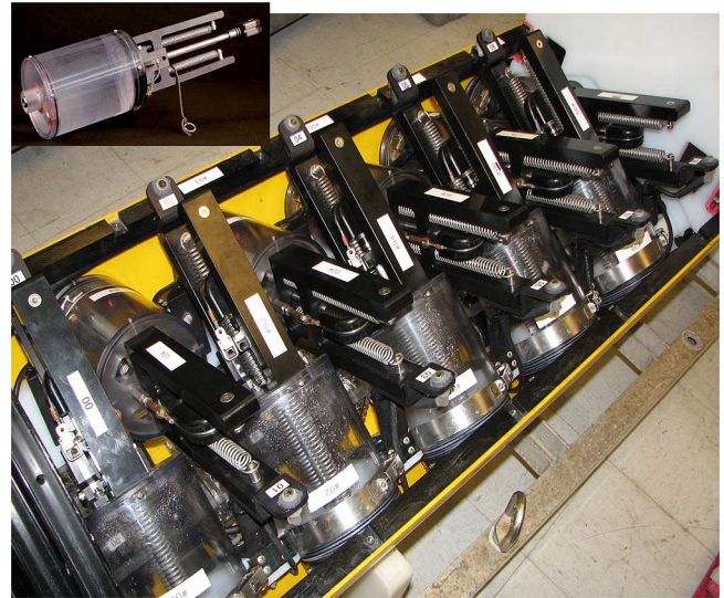
Fig. 1. The ten gulpers on the Dorado AUV (courtesy of L. Bird and A. Sherman of MBARI).
