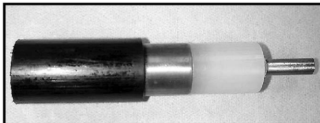
Fig. 2. Photograph of a piece of cable similar to the ATOC/Pioneer Seamount cable. The 3.2 cm wide, coaxial Type SD cable has been cut open to expose interior sections. The cable has a copper inner conductor that contains steel wires, a white polyethylene insulating material, an outer copper sheath, and a black, high-density polyethylene jacket. Cable specification information from University of Washington (1995). Sample courtesy of UCSD-SIO.
