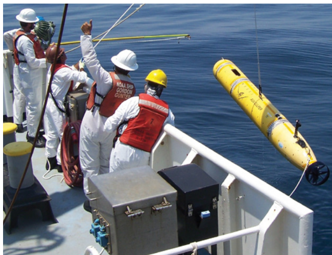
Figure 23. Recovery of the Dorado AUV following a mission in the Gulf of Mexico.
