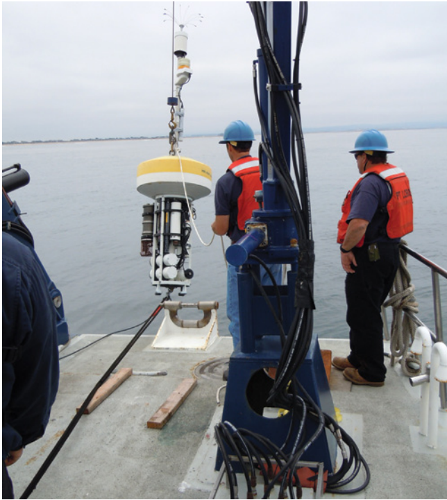
Figure 2: A LOBO mooring is deployed from the R/V Zephyr one kilometer offshore. The mooring carried seven different pH sensor systems for a test of anti-fouling protection schemes during summer and fall 2010.
