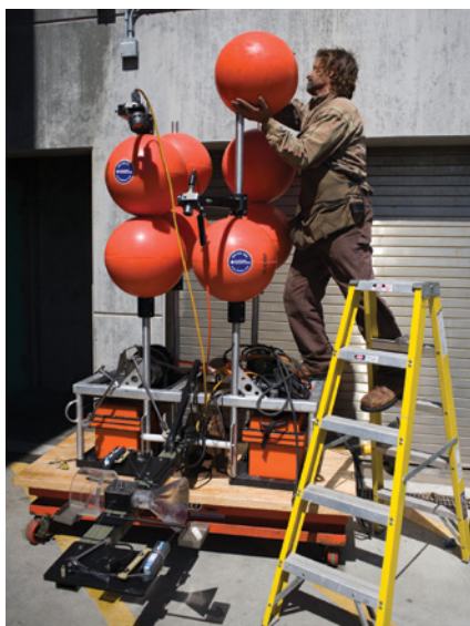
Larry Bird works on construction of an automated system for sampling animal tissue in the deep sea.
