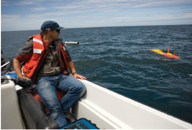
Engineer Brett Hobson prepares for recovery of the long-range autonomous underwater vehicle Tethys at the end of a day's mission during a large October experiment—the first time the vehicle was used for science.
