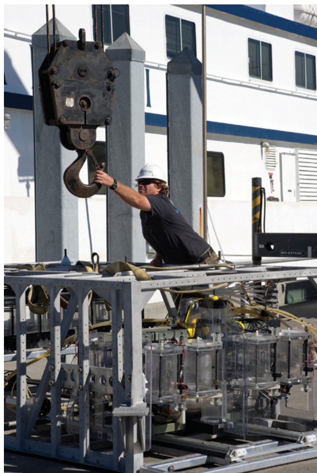
Figure 39: ROV pilot Randy Prickett prepares a toolsled to be lifted onto the R/V Western Flyer , so that it can be attached to the ROV Doc Ricketts for midwater respiration experiments.
