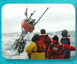
■ The In Situ Ultraviolet Spectrophotometer (ISUS), a sensor that detects chemical elements in seawater without using reagents
