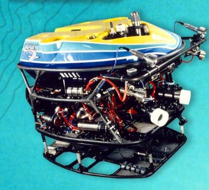
▲ The design and construction of *Tiburon*, a state-ofthe-art, all-electric remotely operated vehicle
