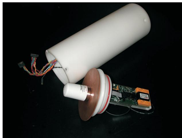
The LOBO radio assembly, shown above, incorporates a MBARI designed interface that provides electrical isolation between the LOBO datalogger and the Cirronet WIT2410 Wireless LAN module. Electrical isolation of the data and control lines minimizes sensitivity loss in the radio due to conducted emissions.
