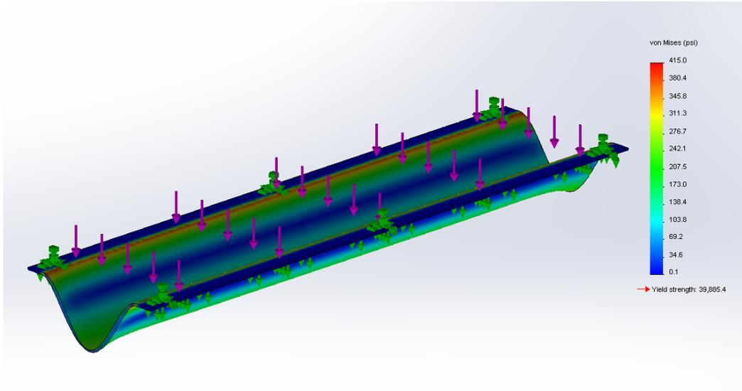
Figure 4: Screen Capture of the SolidWorks Simulation of a 307 lb load uniformly distributed over a 51.5 in x 13.25 in x 0.1875 in 6061 T6 Aluminum rectangular plate with fixed geometries at the 6 hole locations and roller/slider fixture 1.25 inches along each long edge.
