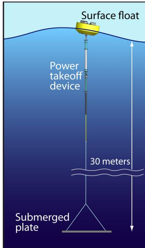
Figure 1: Representation of the deployed PowerBuoy
