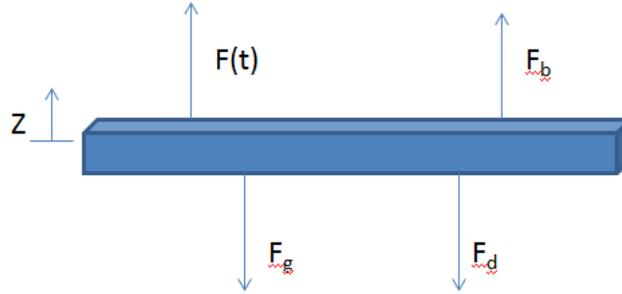
Figure 7: Free body diagram of the Submerged Plate during testing
