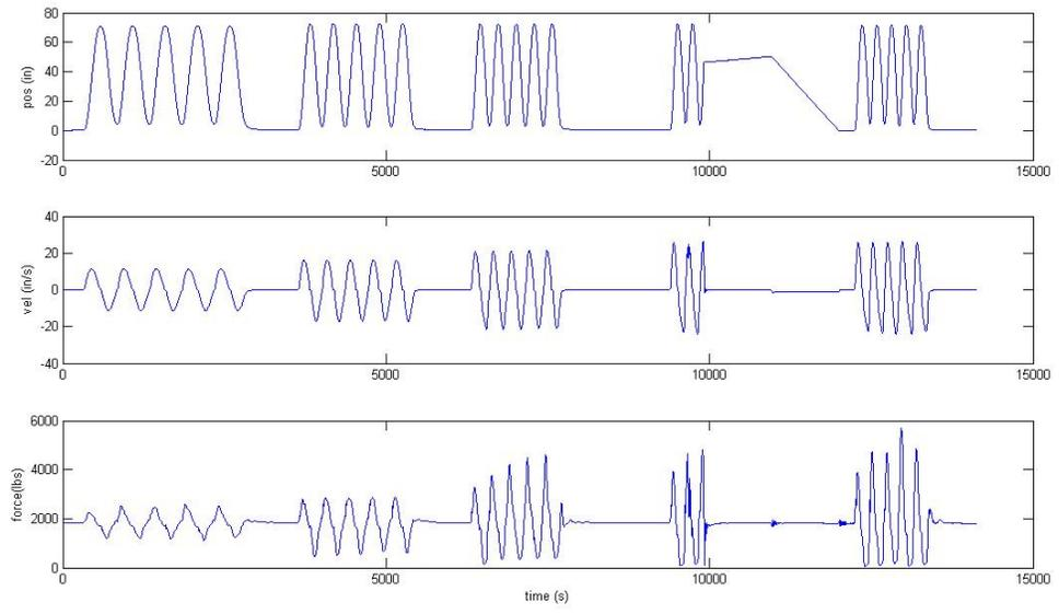
36-Inch Amplitude Test without Plates
