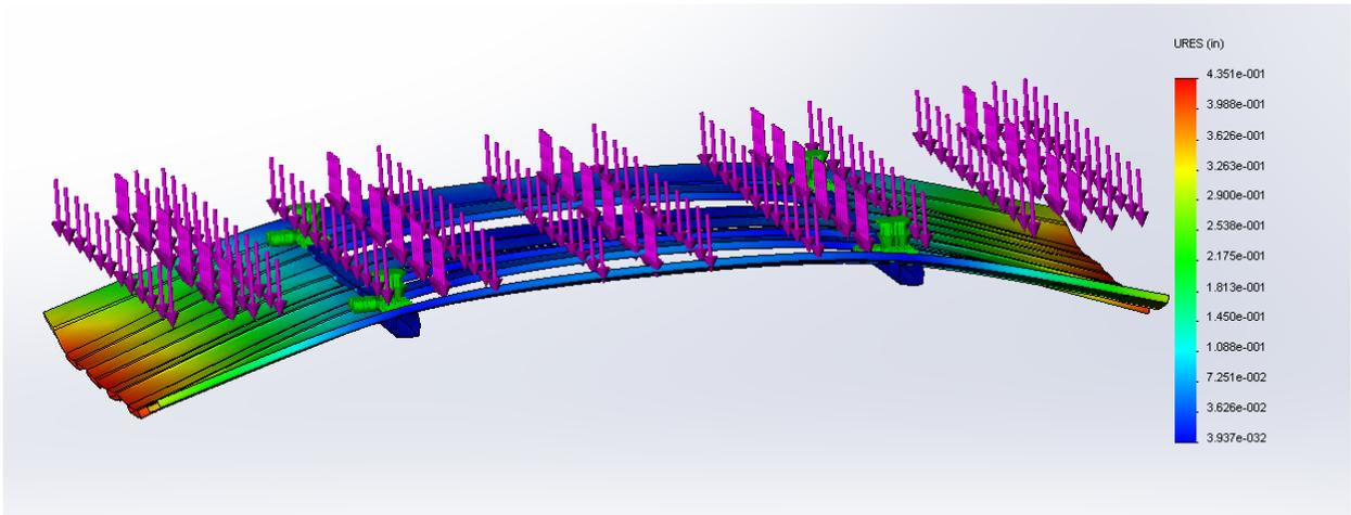
Figure 6: Displacement of Submerged Plate with the 12 Fill-In Plates under a 10000 lb Uniformly Distributed Load
