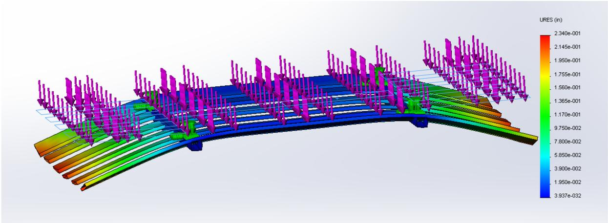
Figure 5: Displacement of Submerged Plate without Fill-In Plates under a 10000 lb Uniformly Distributed Load
