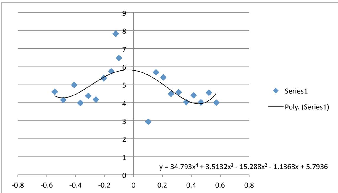
Figure 12:  $C_D$  as a function of speed without the plates
