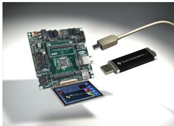
**Figure 2 Stellaris LM3S9B96 Microcontroller Development Kit (DK-LM3S9B96)**
