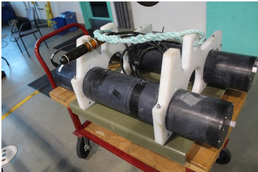
Figure 4. Packed up McSTAR with the fixed hydrophone, electronic container and battery container
