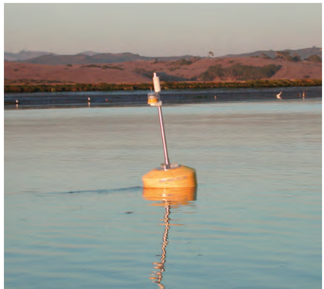
Figure 10: Sensors on this Land/Ocean Biochemical Observatory mooring in Elkhorn Slough record the daily transport of nitrate in and out of the wetland slough.
