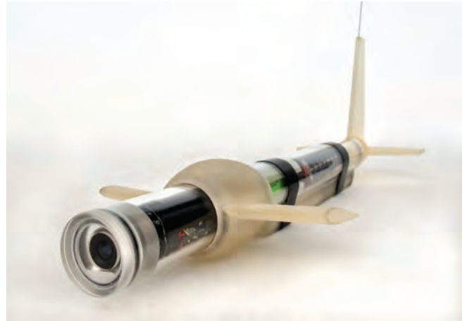
Figure 66: The first functional prototype of the "SharkCafeCam", includes the video camera, battery with solar-energy harvesting, depth sensor, accelerometer, magnetometer, and temperature and light sensors.
