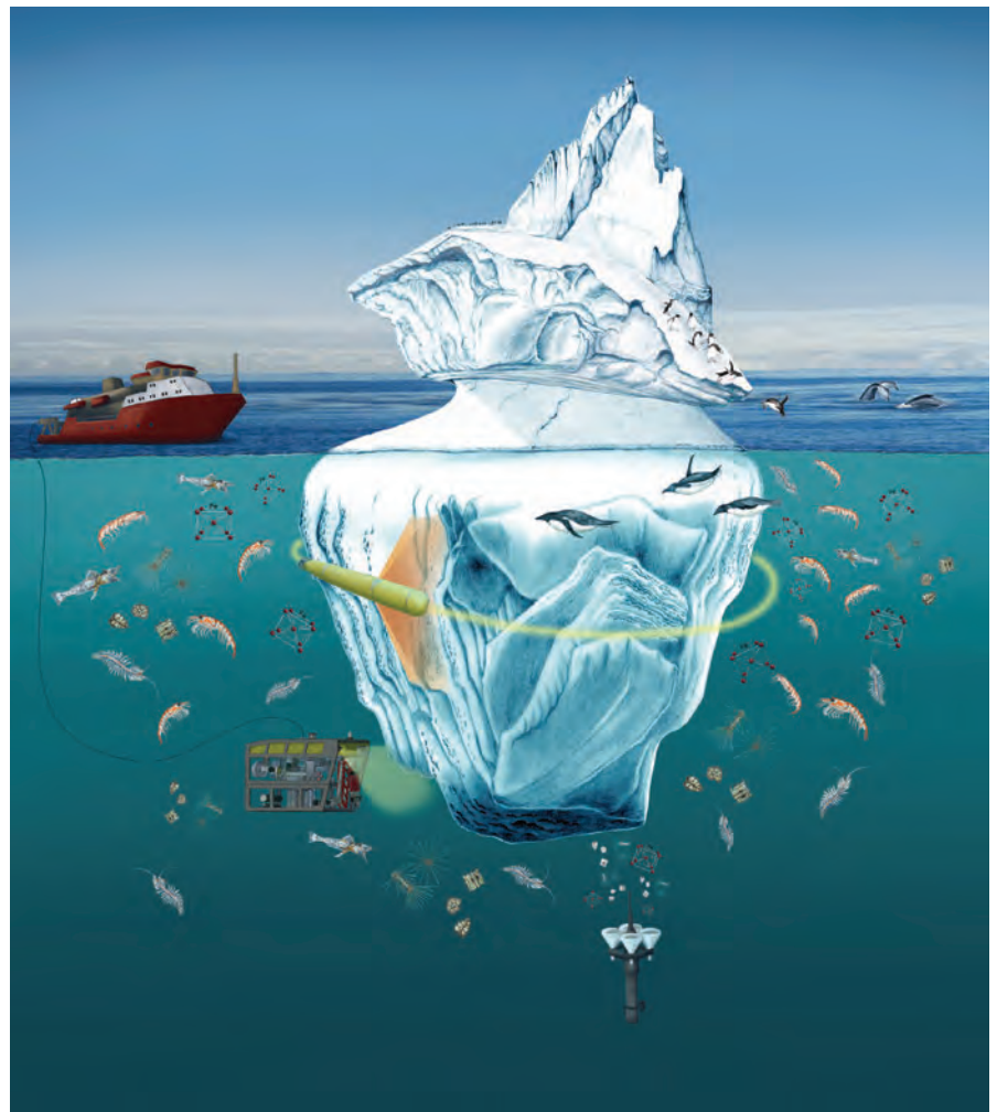
Figure 25: A schematic of the interacting chemical, biological, and physical processes surrounding an iceberg being sampled by a ship, an autonomous underwater vehicle, a remotely operated vehicle, and a Lagrangian sediment trap.
