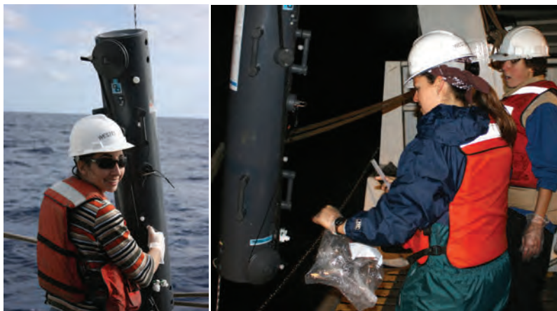
Figure 17: Trace-metal clean-sampling devices are used to target specific algal populations with as little impact to water chemistry as possible. At left, Microbiologist Alexandra Worden prepares to deploy the bottle from the back of the research vessel Western Flyer ; at right, Graduate Research Assistants Melinda Simmons and Darcy McRose prepare for a launch at night during the same cruise.
