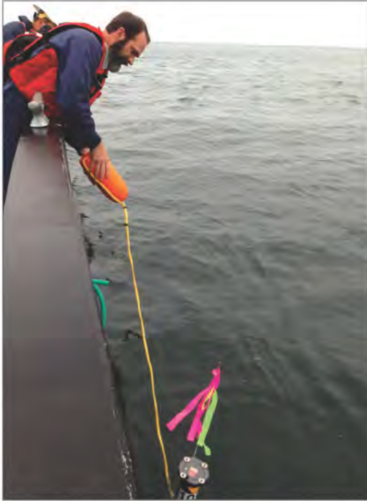
Figure 53: Working from the deck of the research vessel Rachel Carson , Senior Research Specialist John Ryan launches a drifter to study the circulation in San Pedro Bay. The drifter's surface float, which has a GPS that sends its geographic position to shore, is attached to a subsurface drogue that drifts with the ocean currents.
