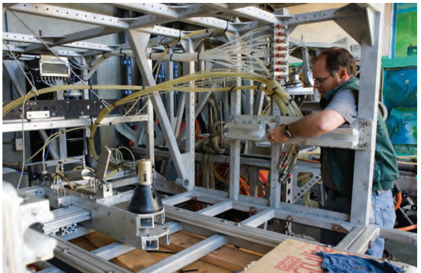
Research Specialist Kim Reisenbichler helped develop the Midwater Respirometry System, which allows in situ experiments on the metabolism of midwater animals.
