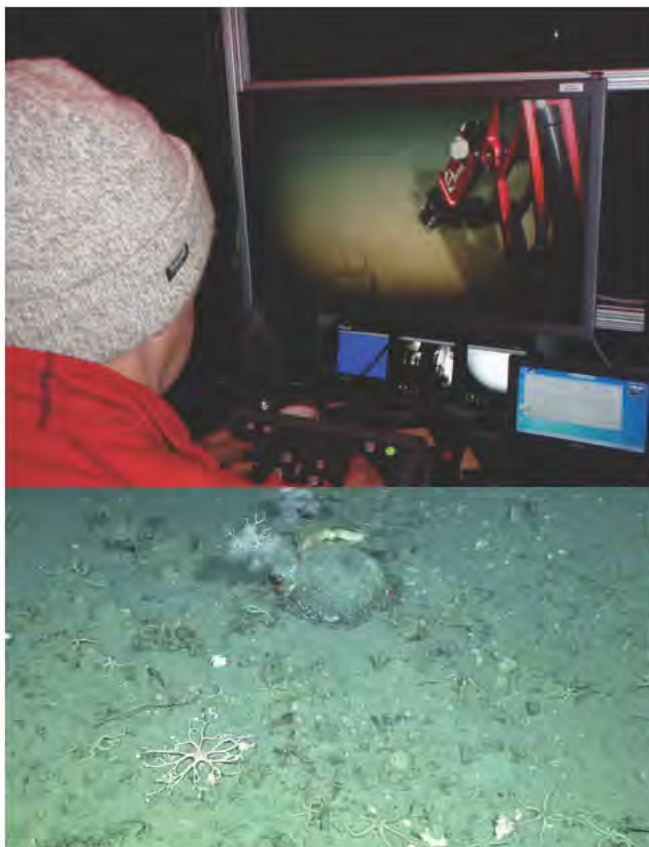
Figure 36: Dale Graves, above, flies the mini ROV and uses its manipulator arm to sample rocks. Still image from video, below, shows a boulder and other rocks scattered on the seafloor that are characteristic of glacial till deposits.
