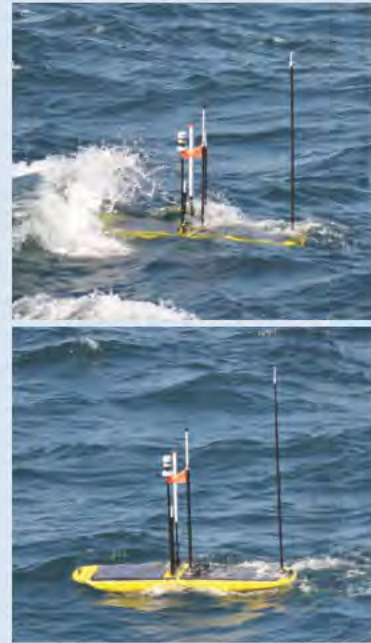
Figure 24: The Wave Glider communications hotspot and the radio relay antennas are designed for harsh ocean conditions. The vehicle's surface float is a little over two meters long.
