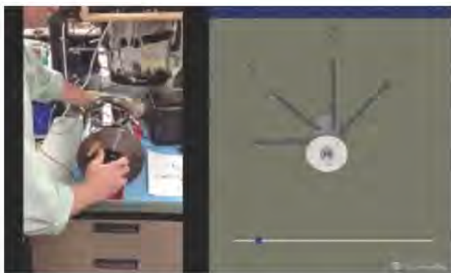
Figure 21: Left, the BED electronic package. Right, software display of BED orientation data.
