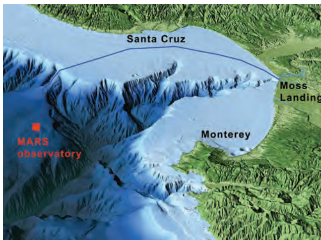
Figure 15: The Environmental Sample Processor was deployed on the Monterey Accelerated Research System cabled observatory, which provides a steady power and communications link to the node at the end of a 52-kilometer cable at a depth of 900 meters below the sea surface.
