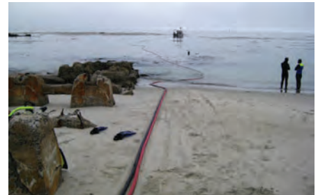
Hoses to supply carbon-dioxide-enriched seawater to the Free Ocean Carbon Dioxide Enrichment equipment stretch across the beach in Pacific Grove, California, and out to the shallow-water FOCE site.
