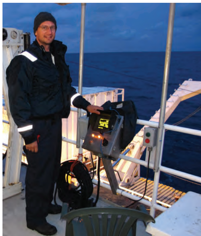
Figure 39: Deckhand Jason Jordan operates the winch from the upper deck of the R/V Western Flyer for evening seafloor sampling. Heavy metal cores with wax-filled steel buds on the end are dropped to the seafloor. Upon impact with the submarine volcano, the cores chip off small bits of volcanic glass which stick to the wax. Laboratory analyses of these bits of glass provide clues to the age of the lava flow.
