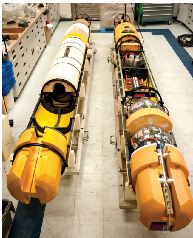
Figure 49: A side-by-side view of MBARI's two deep-water mapping AUVs. The original vehicle is shown on the right, configured for benthic-imaging surveys. The new vehicle, shown on the left with syntactic foam modules in place, is designed for depths as great as 6,000 meters.
