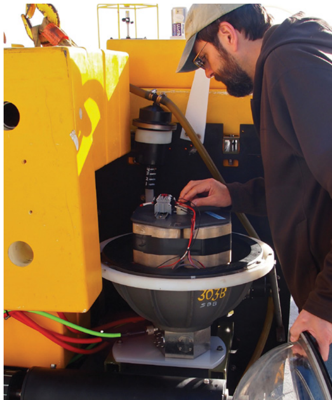
Figure 5: Engineer Paul McGill checks the Benthic Rover's battery pack after its retrieval.
