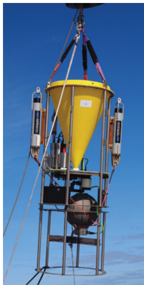
Detritus collected with this Sedimentation Event Sensor is deposited onto a microscope slide, which is then photographed in situ.
