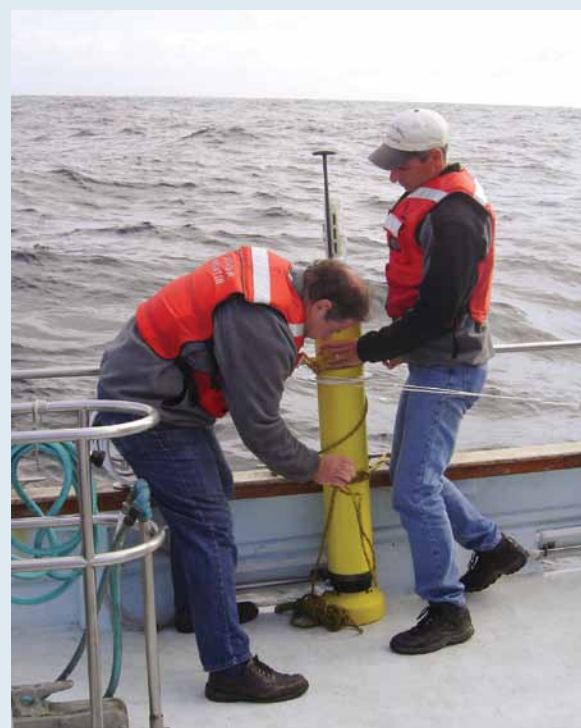
An Apex float fitted with an In Situ Ultraviolet Spectrophotometer is prepared for deployment.
