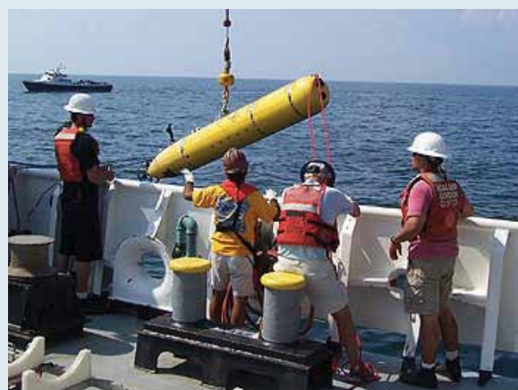
Launching the upper-water-column AUV from a NOAA ship in the Gulf of Mexico.
