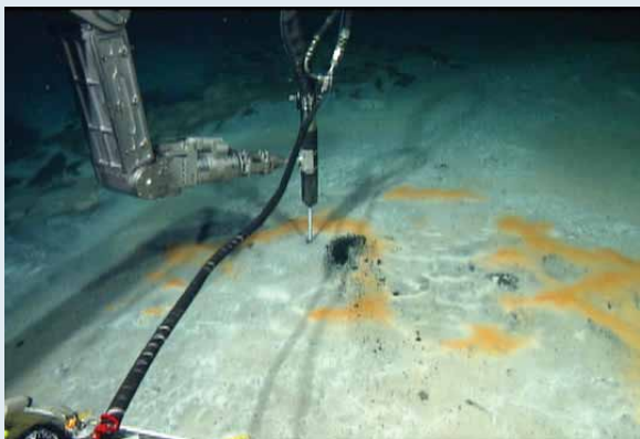
The ROV inserts a laser Raman spectrometer probe into the seafloor to take in situ measurements of this methane-rich area covered in bacterial mats.
