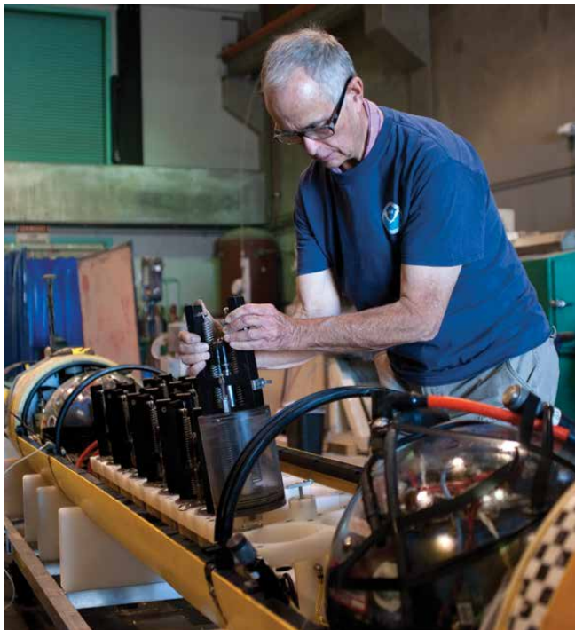
Figure 5. AUV Operations Engineer Duane Thompson sets a gulper water sampler into the AUV for a mission in Monterey Bay.
