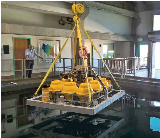
Figure 47: MBARI Geologist Charlie Paull watches as an array of instruments (a benthic instrument node) is lowered into MBARI's test tank in preparation for being placed on the seafloor during the Coordinated Canyon Experiment.
