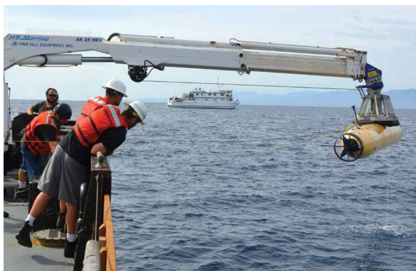
Figure 14. The mapping AUV is recovered to the R/V Rachel Carson after the ROV Doc Ricketts , aboard the R/V Western Flyer (in the distance), was used to cut it free from a derelict fishing line. Part of the line can be seen still attached to the AUV antenna.
