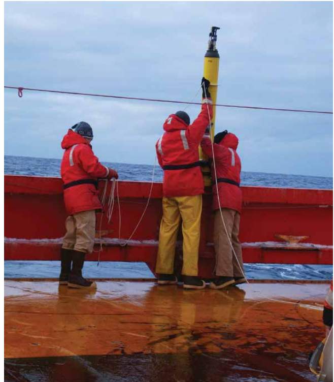
Figure 11. SOCCOM scientists deploying a profiling float from the R/V Palmer in the Southern Ocean in 2014.
