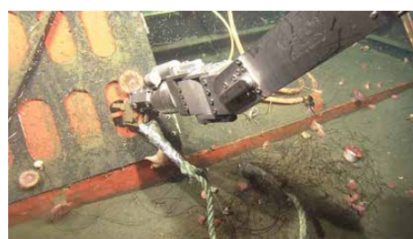
ROV Ventana's robotic arm disconnects a shackle during the placement of a hydrophone on the MARS observatory.
