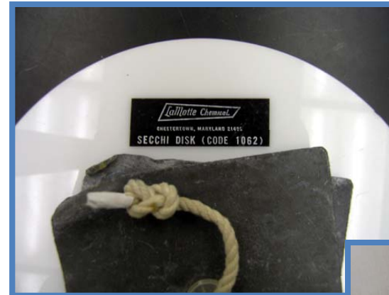
Left: A Figure 8 knot is used on the bottom of the secchi disc to secure the disk to the rope.
