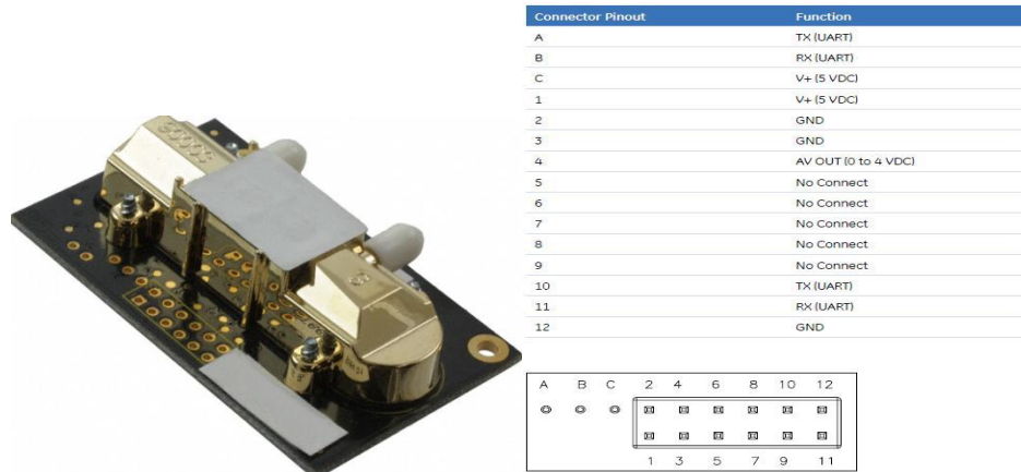
Figure 7 ( picture of the Telaire T6615F along with the Pinout description)
