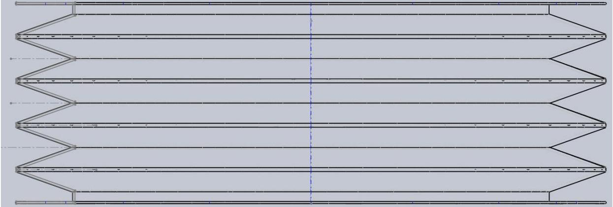
Figure 8 – The above sketch shows the idealized geometry of the bellows.
