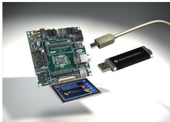
**Figure 2 Stellaris LM3S9B96 Microcontroller Development Kit (DK-LM3S9B96)**
