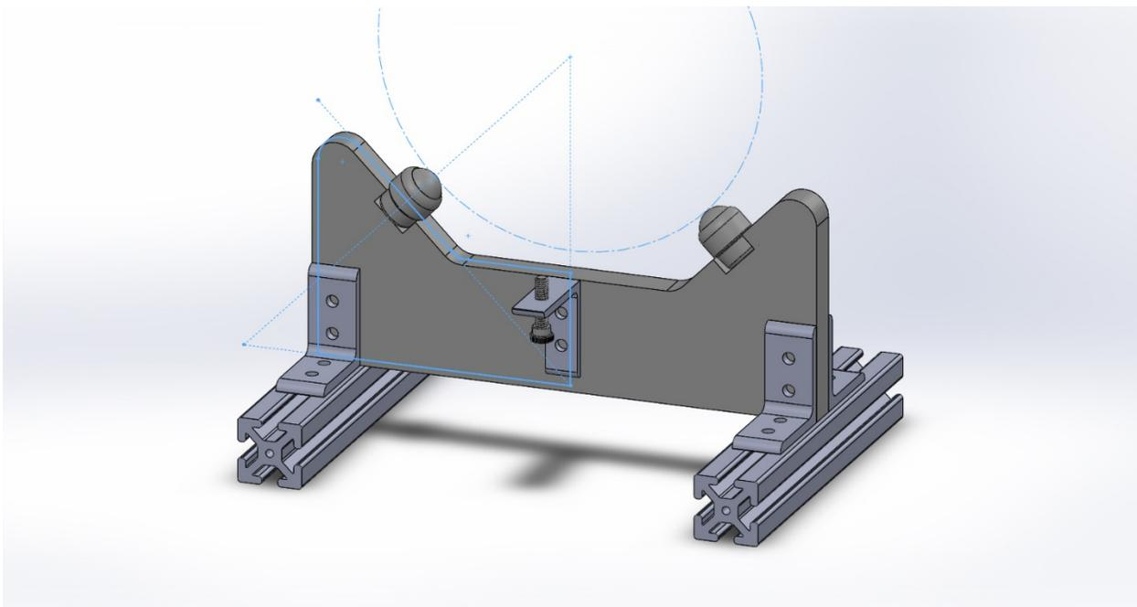
Fig 5: LRAUV Support Chock assembly, used to support the LRAUV on the floor scales
