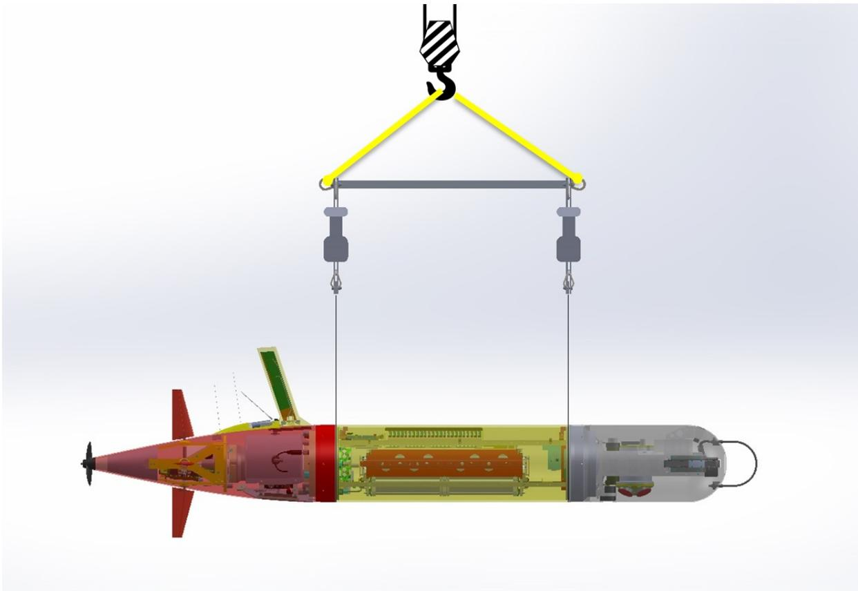
**Fig 2:** MBARI's LRAUV on a dual hung scale design to measure center of gravity
