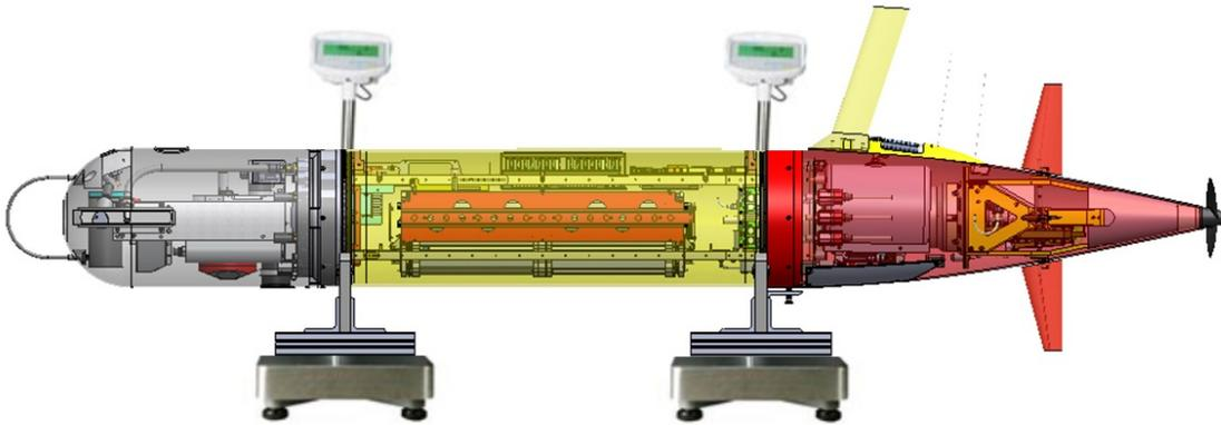
**Fig 3:** MBARI's LRAUV on a dual floor scale design to measure center of gravity
