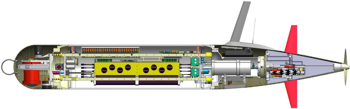
**Fig 1:** Cross sectional view of MBARI's LRAUV
