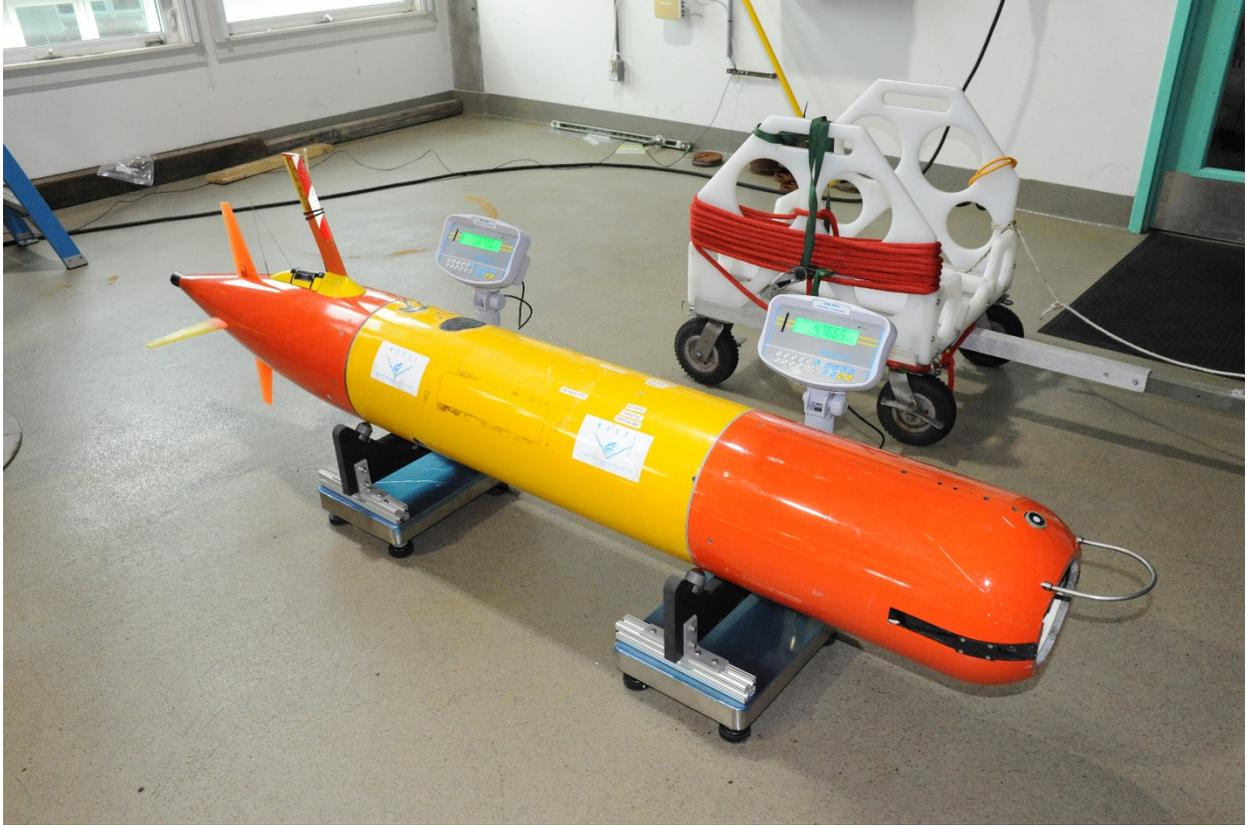
**Fig 8:** LRAUV Procedure application using Vehicle supports and scale system.
