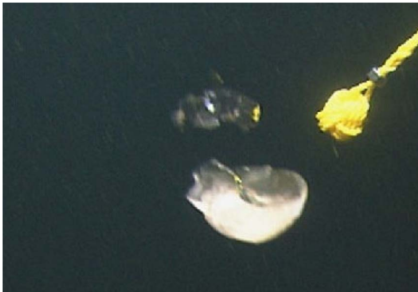
Fig. 4. A CO 2 slurry mass sinking at around 0.3 m/s.
