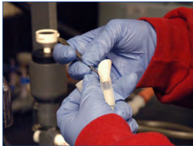
Figure 4. Filter, sample side in, being placed in cryovial for archival and/or lysis.
