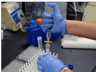
Figure 6. After lysis, lysate is syringe filtered into clean tube.
