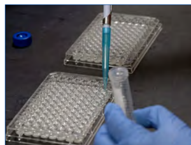
Figure 7. Lysate (0.25 mL) is added to appropriate sample wells on microplate.
